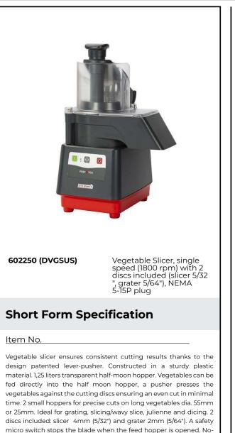
micro switch stops the blade when the feed hopper is opened. Novolt release system prevents accidental start of the appliance. All parts in contact with food are removable and Dishwasher safe. Single speed 1800 rpm with on/pulse/off function for simple operations. NEMA 5-15P plug
